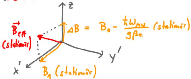
Beispiel 1:  $\Delta B = 0$  ( $\omega_{MW} = \omega_L$ , on-resonance)
